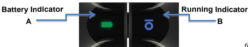
**A. Battery Indicator:** The Green LED light indicates the IO HAWK is charged >50%, the Yellow LED light indicates the power is under <50%, the Red LED light indicates the power is down to 10%, when the LED light becomes red, please recharge the device.
